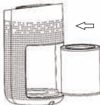
⑤ Insert the new HEPA filter into the 49200. Open side facing up
