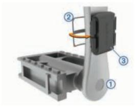
4 Rotate the crank arm to check for clearance.
