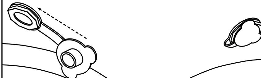
Press the rubber drain plug firmly before filling the bath bucket with water. First fill the bath bucket with a small layer of water to check that no water is leaking.
