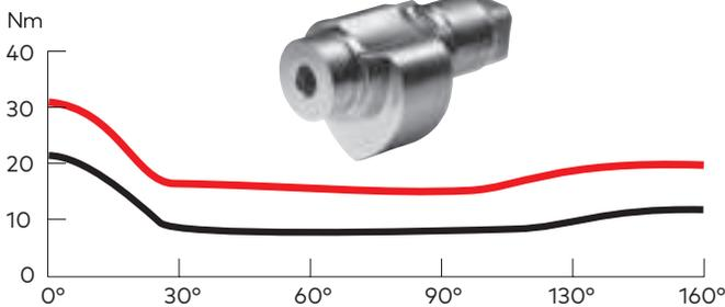
The unique heart-shaped cam and the linear drive mechanism ensure that the resistance encountered decreases almost instantly with the door opening action.
