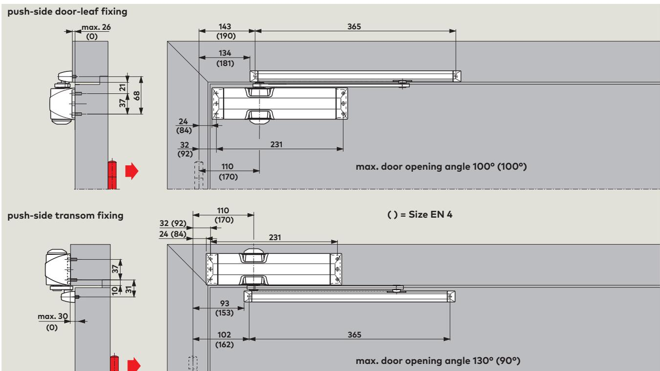
Depending on the structural conditions, the door opening angle is likely to be limited to approx. 95°. It is recommended to install the cushioned limit stay or position a door stop at this point. As the door opening is limited to 95° the TS90 is not CE marked on the push side of the door. BS EN1154 requires minimum closing from 105°.
