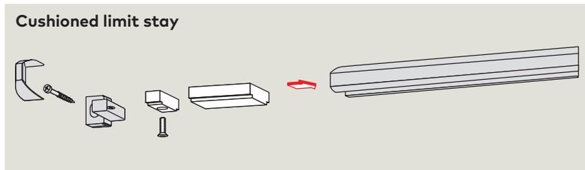
Cushioned limit stay for retro fitting by insertion in the slide channel. Adjustable between 80° and max. 120°.
