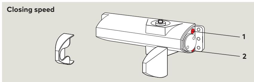
The closing speed of the TS 90 Impulse is adjustable in two independent ranges at the valves indicated.
