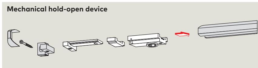
The hold-open device enables doors to be precisely held without any fall-back up to an opening angle of approx. 145°.
