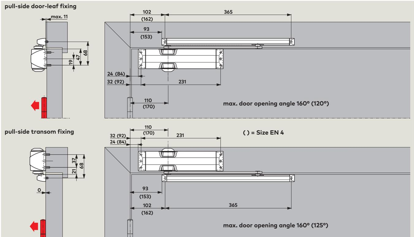
Depending on the structural conditions, the door opening angle is likely to be limited. It is recommended to install the cushioned limit stay or position a door stop at this point. **A door stop must be installed in the case of fire and smoke check doors.**
