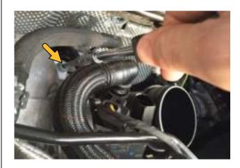
Rotate the top of the intake elbow towards the firewall to disengage it from the turbo.
