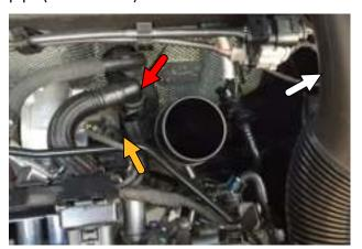
Using a Torx T30 driver, loosen the single screw (yellow arrow) that retains the hard plastic turbo intake elbow. This screw usually has an o-ring under it to prevent it from falling out as it is loosened, but take care not to drop it anyway.
