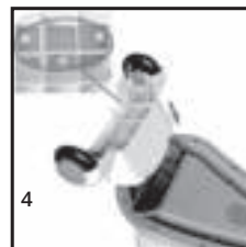
Figure 4: Install the rear wheel assembly (part 5) into the body (part 1) and fasten the buckle. Then install three screws (part 3) into the bridge of the rear wheel (part 5) and tighten them.
