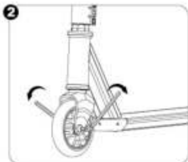
Securely tighten the bolt as shown.
