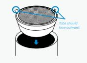
Unwrap the new filters and place them into the housing with the pull tabs facing out.
