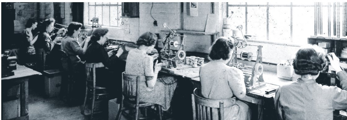
Winding coils for Marconi transformers kept the 20 staff busy throughout the war.
