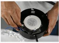
3, connect the wire of the light to the motor, pay attention to the proper side
