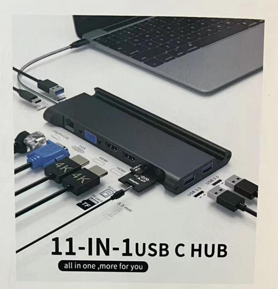
3\*USB3.0+2\*HDMI 4K+SD/TF+RJ45 gigabit +3.5 Audio/Mic+USB-C PD charging
