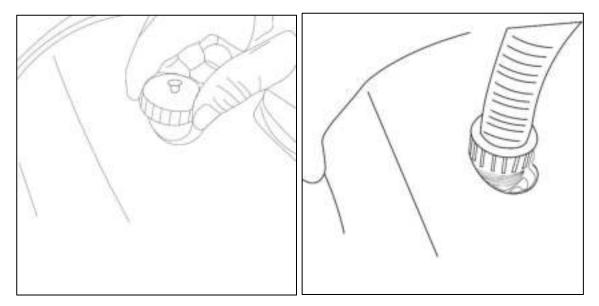
• c. Open the air valve on the whirlpool cover and attach the filling hose to the valve.
