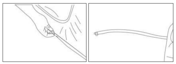
Then pull off the plastic plug on the inside. Now the water can flow out. When the spa is out of water, press the BUBBLE button for 2-3 minutes to drain the water in the air line.
