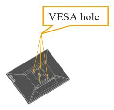
Step 5: Attach the LCD display to the wall, following the instructions in the wallmounting kit. For use only with UL/GS Listed Wall Mount Bracket with minimum weight/load: 13.86 kg
