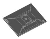
Step 4: Attach the mounting bracket from the VESA compatible wall mounting kit (100mm x100mm distance), VESA Mounting Screw M4 x 10 mm.
