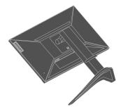
Step 3: Remove the base from the monitor, refer to "Detaching the monitor base and stand".
