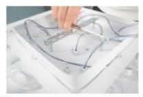
10, put down the cross, make sure all the screws can go through the four small holes at the plate, then take it out and fasten the nuts
