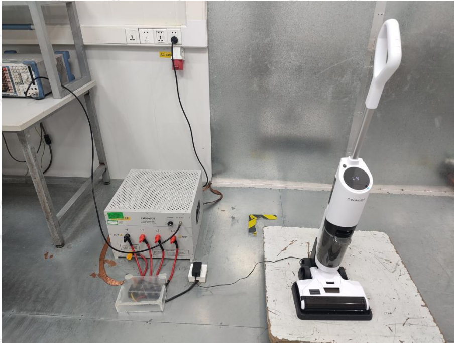
Photo of Power Line Conducted Emission Test
