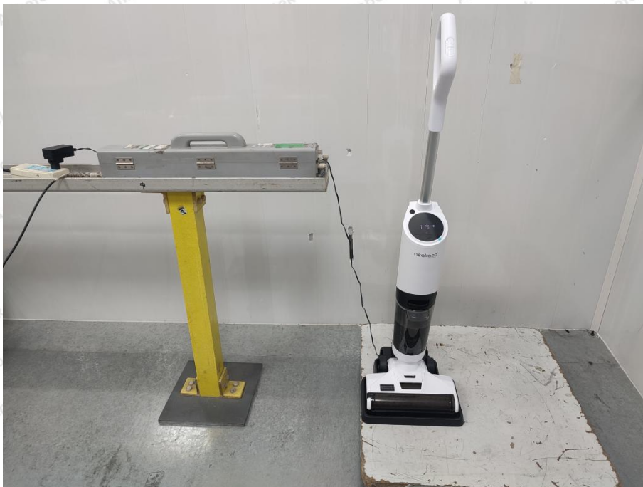
Photo of Disturbance Power Test
