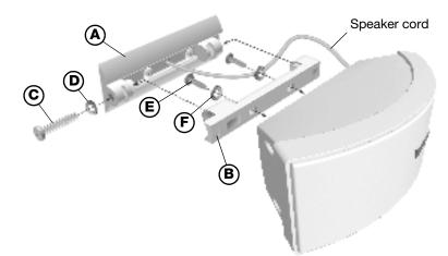
2. Hold bracket part **A** in position against the wall and mark the left and right round holes for the mounting hardware (Figure 4). If you plan to feed speaker cord through the wall, mark the oval speaker cord feed-through hole also.
