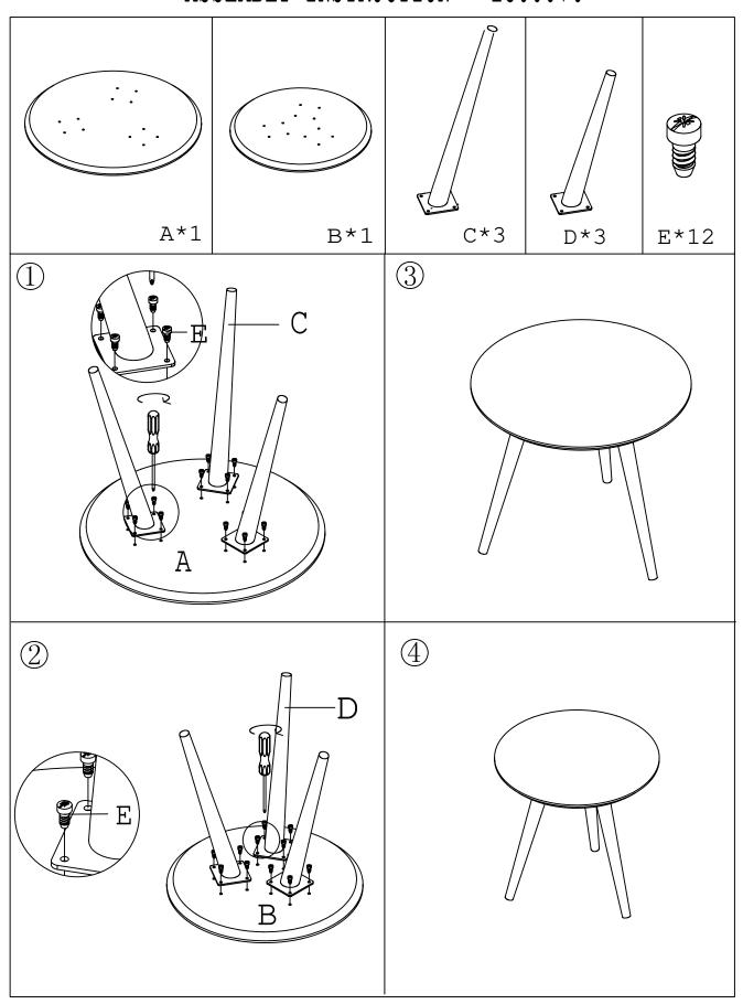
Do not tighten the screws completely until all screws are connected.
