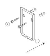
**SCREWS FIXING** Fix the back panel(1) of the dock to the wall using the screws(2) included.
