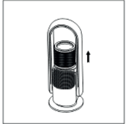
Lift out the old air filter
