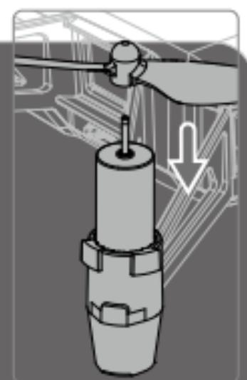
Mount unmarked propellers on the motors with unmarked landing gear.
