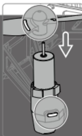
Mount marked propellers on the motors with marked landing gear.
