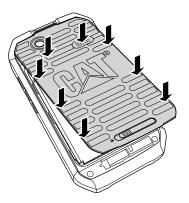
4. Press and hold the bottom of the back cover and slide the back cover latch to the left to the lock the back cover.
