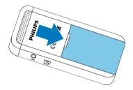
Insert the batteries or rechargeable batteries into the device as shown. Make sure the polarity is correct.
