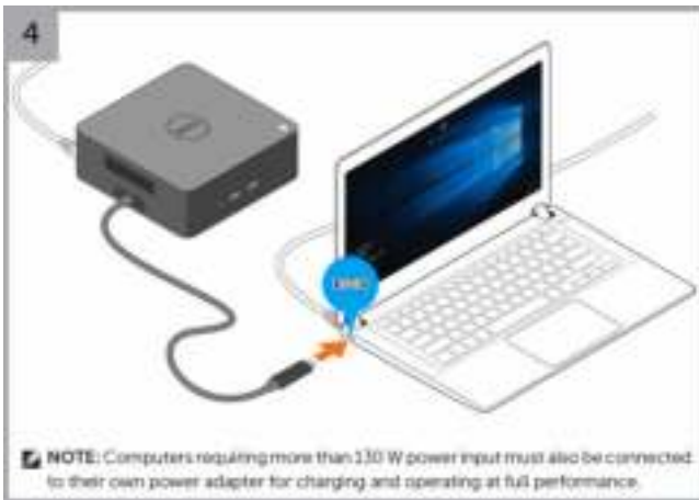
Figure 4. Connecting the Thunderbolt 3 (Type-C) connector
