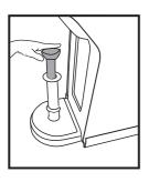
Step 3#: inject the water from pipe into the machine so that the internal circuit is filled with water.
