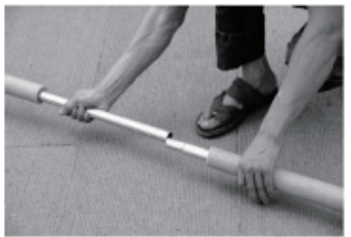
Insert the end cap on the upper tube and the end button on the bottom stand rod. Then slide the rods together.
