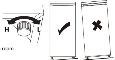
Do not place the appliance near heat sources such as central heating or a stove. Do take note of the climate class of the appliance. When placed in a room that is too cold, the freezer will not function properly.
