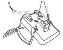
**Step 5:** Attach the seat back and arms to the seat bottom using screws (c, b) and washers (H) as shown.
