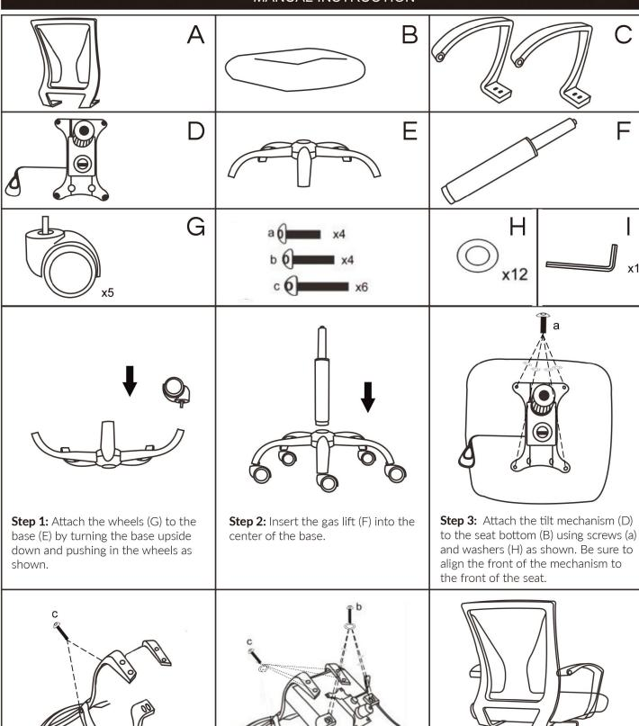
Step 4: Attach the arms (C) to the seat back (A) using screws (c).
