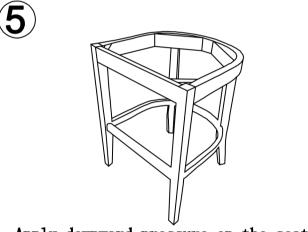
Apply downward pressure on the seat frame to ensure the chair is level before tightening all screws firmly with allen key(tight to 90%)
