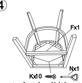
open two front legs lightly, put Fx1 inside then useing Kx10, hand tighten to 80%
