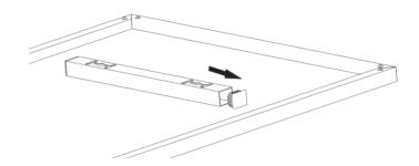
4. Slide the panel to make ceiling hanging units into one side of the panel rear first, then push the whole panel close to ceiling and slid the panel back, to make the other two hanging units into the other side of the panel.
