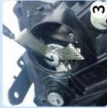
Insert the headlight and screw tight to clockwise direction
