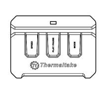
SPEED: Switch over between 2 fan speed modes LED Indicator shows Blue: Normal mode 800~1500rpm LED Indicator shows Red: Low noise mode 400~1000rpm
