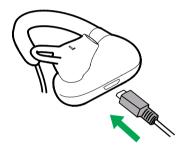
It takes approx. 2 hours to fully charge the battery. If the earbuds are fully out of battery, 15 minutes of charging will give 1 hour of battery.
