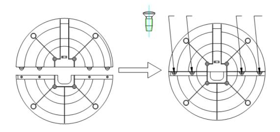
3. Pass the power cord through the bottom panel, and insert the base plate with four screws and the main body of the product.
